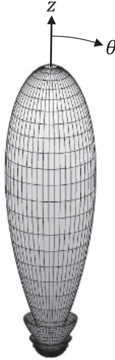
FIGURE 6.27 3D total field pattern of a dish antenna with aperture size a = 5\lambda .
